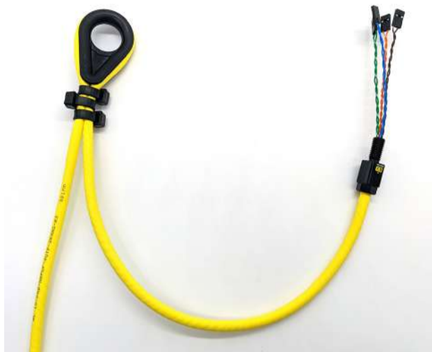
Regular Fathom Tether wrapped around the thimble.
